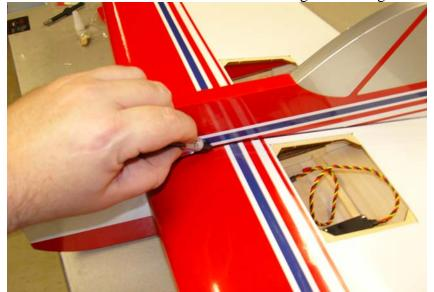
13. Remove the wing from the fuselage and use an old soldering iron or sharp hobby knife to remove the covering from the center of the wing. Use some denatured
