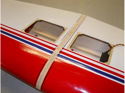
14. Slide the wing into position just a few inches short of its proper location. Mix up some 30 minute epoxy and apply to the exposed wood at the center of the wing with an epoxy brush.
