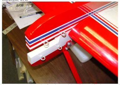
33. Secure the tank to the fuselage with nylon cable ties or rubber bands. Be sure to place a piece of closed cell foam between the tank and fuselage side.
