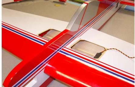
16. Locate the 2 ailerons, 2 composite control horns and 2 base plates. Open the covering over the slot on the bottom of the aileron and insert the control horn into the base and into the slot. Use a fine tipped felt marker to trace the base plate and remove the covering from this area.
