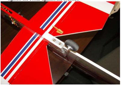
12. Next slide the wing into position and check alignment with fuselage and horizontal stab. Measure to insure wing is positioned properly and then use a fine tipped felt marker to mark the area where the covering will need to be removed to insure a wood-to-wood bond between the wing and fuselage.
