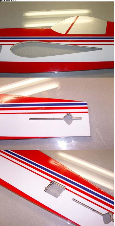
2. Now let's install the horizontal stab and elevator. First insert the stab into its slot in the rear of the fuselage. Use a ruler to assure the stab is centered and a square to make sure it is aligned 90 degrees to the fuselage. Sand or shim the slot as needed to insure proper alignment. Once satisfied use a fine felt tipped marker to scribe the covering where it will need to be removed from the stab to allow a wood-to-wood bond between the fuselage and stab.
