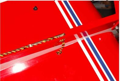
27. Locate the provided strip of Ultracote and iron it into position on the bottom of the fuselage.
